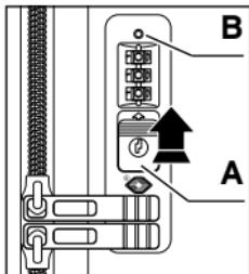
1. Set the combination to the factory default number. To test it, check whether the opener **A** can be pushed up. While setting the new combination leave the zip puller outside the lock.
